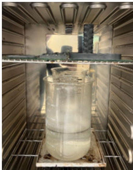
Figure 3: Thermal cure oven with water tank and Silicone parts
