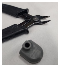
Figure 2: Cutter for removing support
