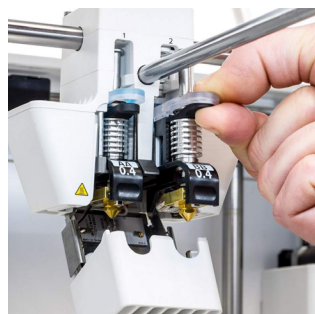
Print core BB Quick-swap nozzles for build and water-soluble support materials. Available in 0.25, 0.4, and 0.8 mm
