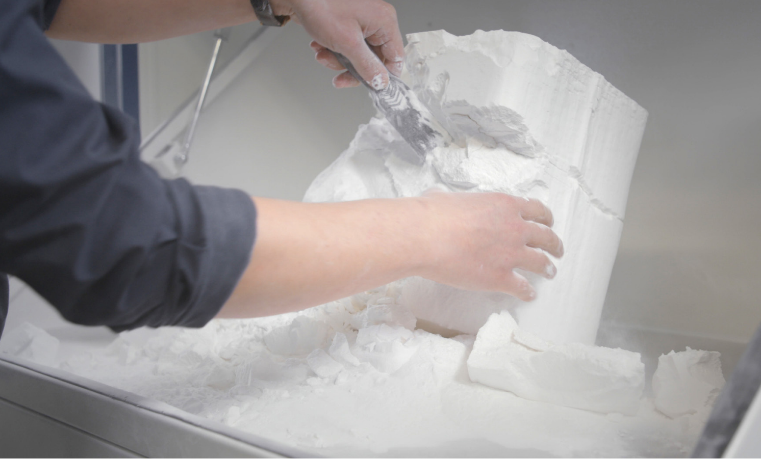
The H350 uses an infrared sensitive HAF™ to fuse particles of polymer powder together in layers to build parts
