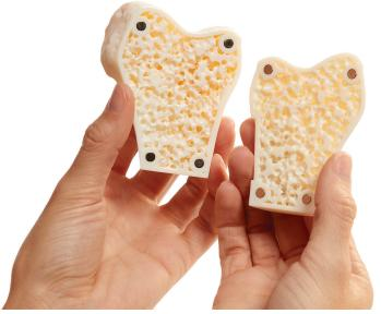
The cancellous bone model demonstrates the ability to replicate complex anatomical structures using GrabCAD Voxel Print. This utility lets medical professionals create models that offer greater realism when practicing procedures like cutting, reaming and drilling, with a performance unobtainable by other modeling methods.
