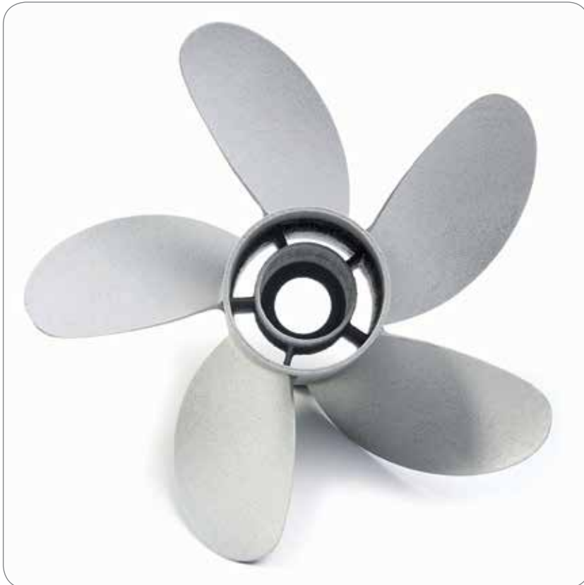
Propeller for racing boats as a scaled model for flow measurements
