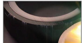
*The Objet500 Connex 3D Printer can build a rubber tire and rigid wheel rim in one piece.*
