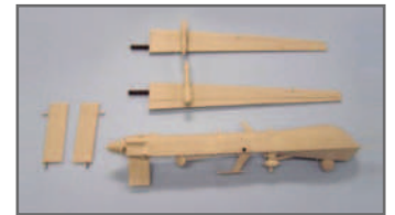
UAV replica fuselage and wings, manufactured with the FDM process.
