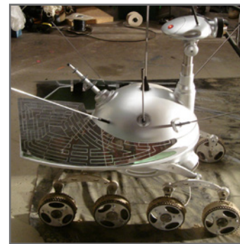
Special effects designers at Artem built this moon buggy prop for a BBC advertisement using parts created with a Dimension 3D Printer.
