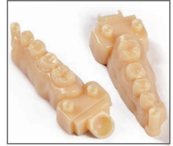
Apex uses an Objet Eden 3D printer to make crowns, bridges, inlays, etc.
